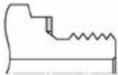
Sealing by compression against face of body Reference DIN 3852 Type A
