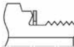
Sealing by gasket (washer) Reference DIN 3852 Type B
